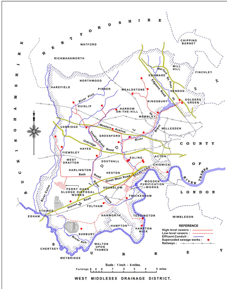
**Figure B-1 Schematic of the West Middlesex Drainage Board plans for Mogden WwTW (after J. Timms)**
