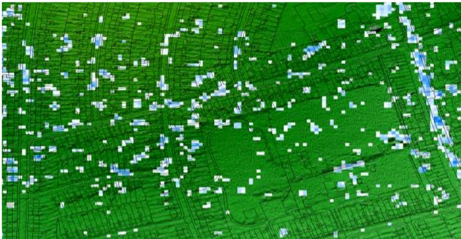
**Figure C-9 LiDAR anomaly caused unusual TUFLOW model outlines**
