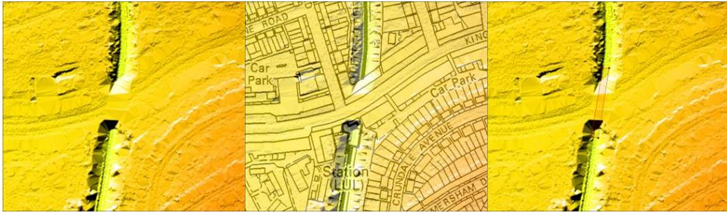
**Figure C-7 Poorly filtered structures in Group 2 LiDAR**
