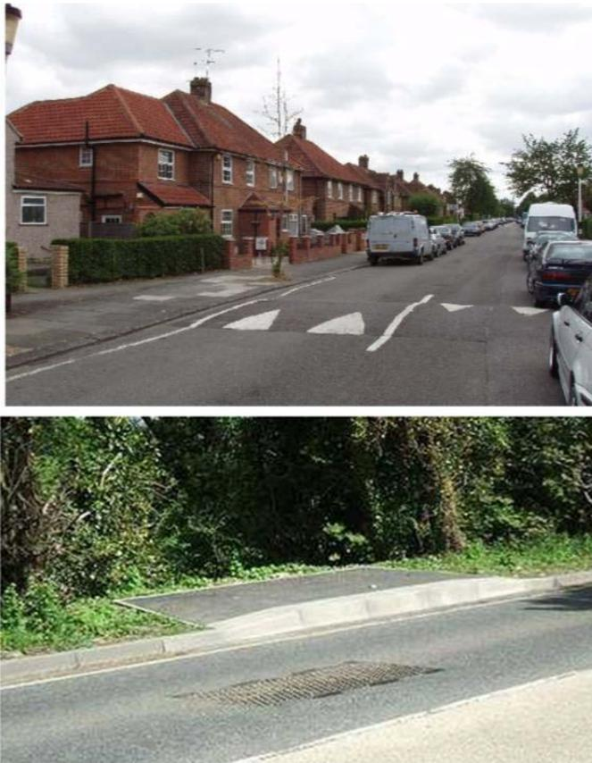
Figure E2-11 Example of a speed hump (Geograph, 2011<sup>ix</sup>) and of raised kerbing (Barkingside, 2009<sup>x</sup>)
